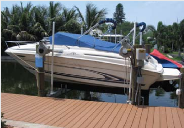
12,000 lb. capacity (4) motor beamless “GatorVator” boat lift with “E-Drives” and remote control
