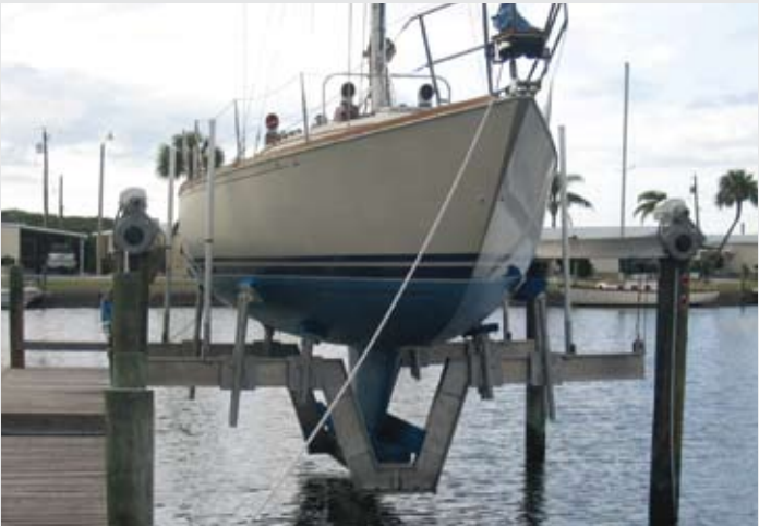
24,000 lb. capacity conventional 4-post boat lift with “E-Drives” and custom bottom cradle beams and bunks
