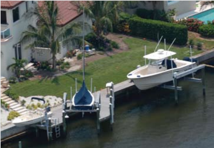
Custom configured marginal dock with composite decking, 24,000 lb. capacity conventional lift, 7,000 lb. capacity sailboat lift and 1,500 lb. capacity PWC lift
