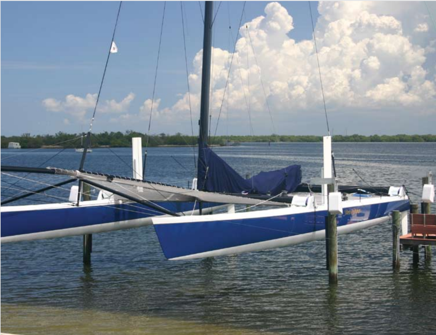
24,000 lb. capacity custom designed lift to accommodate a 78’ sailboat
