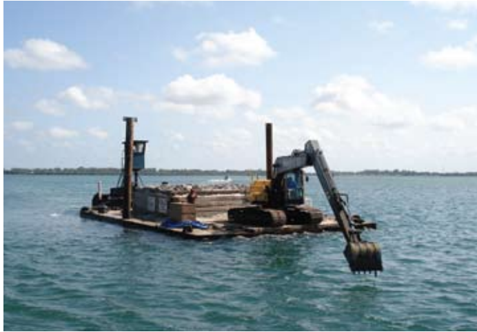
60' dredge barge with long reach track hoe and 120 cubic yard container on the deck
