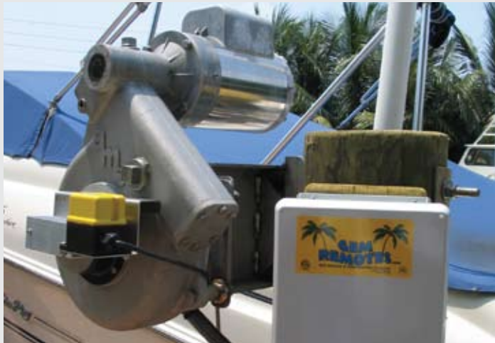
Remote control with limit switch mounted on “E-Drive” and stainless steel motor
