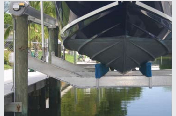
Shallow water (angled) cradle beams
